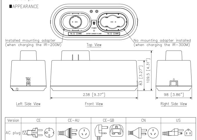
Note: The figure above shows the IR-200BC with one of the mounting adapters removed.
